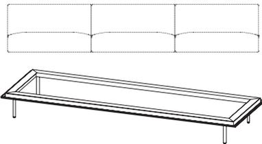
Structural sofa frame made of extruded aluminum profile with 4 legs made of steel rod. The legs can be assembled in different positions.
