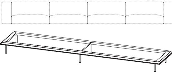
Structural sofa frame made of extruded aluminum profile with 6 legs made of steel rod. The legs can be assembled in different positions.
