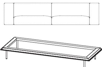
Structural sofa frame made of extruded aluminum profile with 4 legs made of steel rod. The legs can be assembled in different positions.
