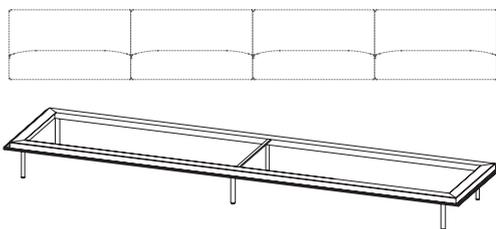
Structural sofa frame made of extruded aluminum profile with 6 legs made of steel rod. The legs can be assembled in different positions.
